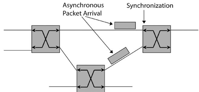
Fig. 1. Packets arrive asynchronously to optical switches.
