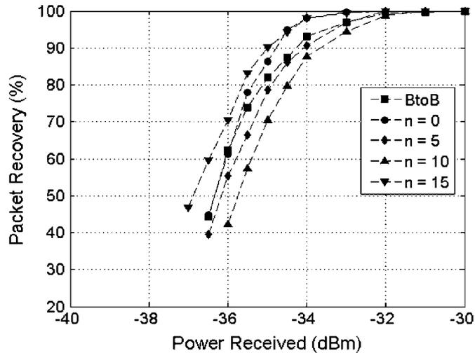
Fig. 8. Packet recovery measurements at input power =  $-11.5$  dBm for synchronizer delays  $n = 0, 5, 10,$  and  $15$ .
