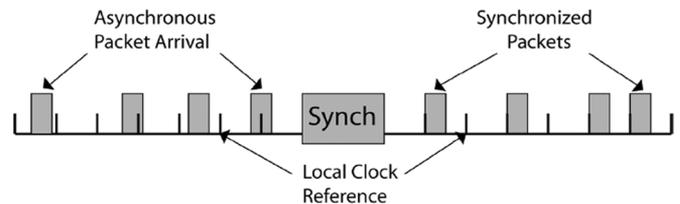
Fig. 2. Synchronization aligns asynchronous packets to a local clock.
