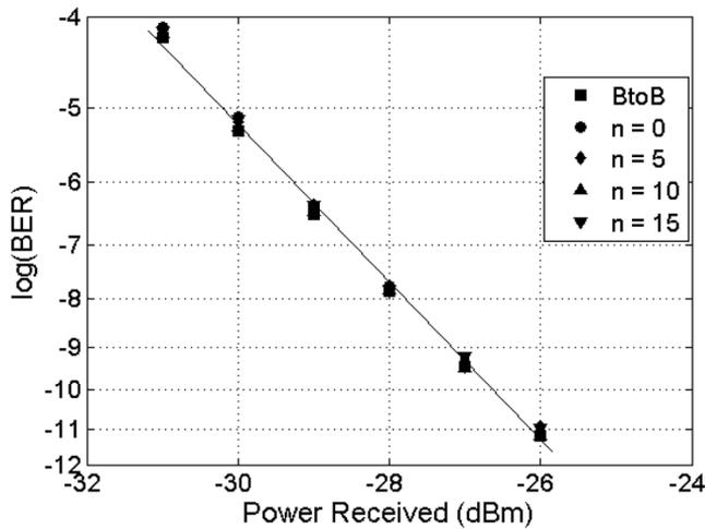
Fig. 4. Layer-1 (BER) measurements at input power =  $-7$  dBm for synchronizer delays of  $n = 0, 5, 10,$  and  $15$ .
