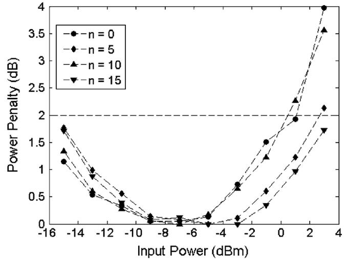
Fig. 5. Input power dynamic range measurements for synchronizer delays of  $n = 0, 5, 10,$  and  $15$ .
