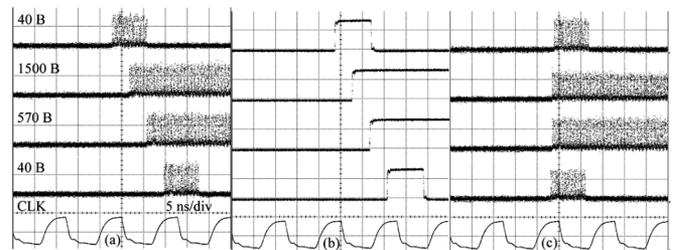
Fig. 7. (a) Asynchronous packets. (b) Recovered payload envelopes. (c) Synchronized packets.
