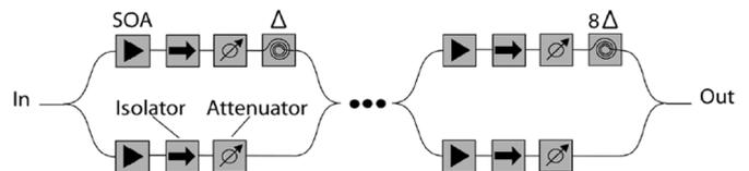
Fig. 3. Fiber-based four-stage synchronizer with SOA gates.
