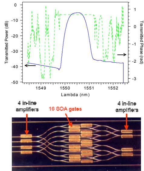
**Figure 2. Measured flat-top pass-band amplitude and phase characteristics (top) and proposed 4x4 integrated optical switch matrix based on SOAs (bottom).**
