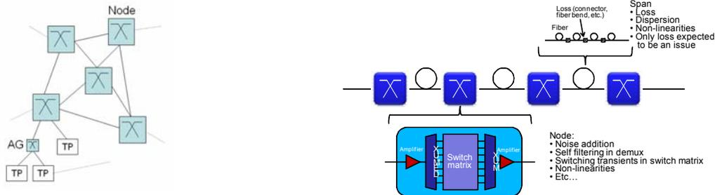
**Fig. 1. Meshed network with interconnected switching nodes and terminations points (TP, end user) and aggregation points (AG) for low traffic volume termination points (left). Reference physical layer path with nodes interspersed by fiber.**
