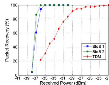
Fig. 6. Packet recovery measurements for back-to-back Tx 1, Tx 2, and TDM packets
