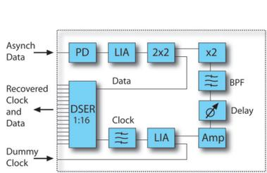
Fig. 4. Schematic of clock and data recovery (CDR) circuit
