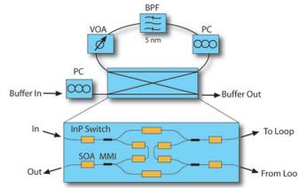
Fig. 2. Re-circulating optical packet buffer with inset of 2x2 InP switch
