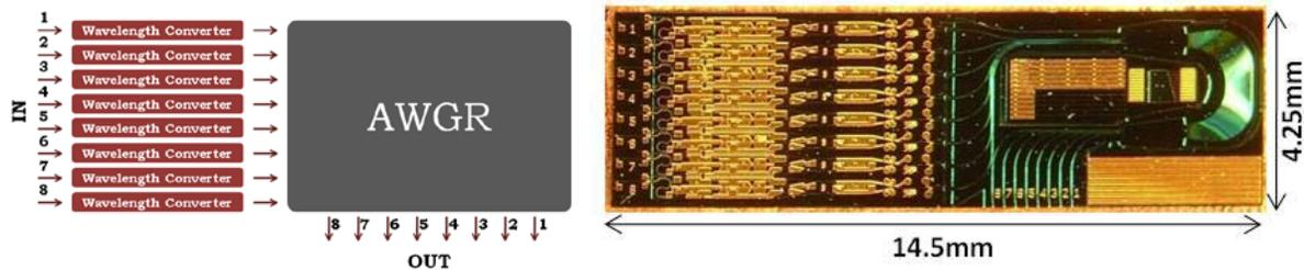
**Figure 3 – (left) Schematic of MOTOR chip (right) Photograph of the fabricated device**
