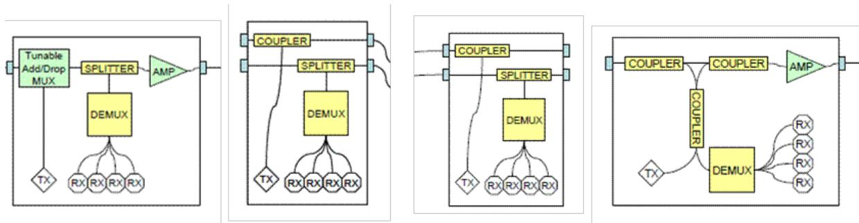
**Figure 1 - Different Connection architectures based on different network topologies: from left to right (1) Ring topology connection (2) Unidirectional bus (3) Star/switch topology (4) Bidirectional bus topology**
