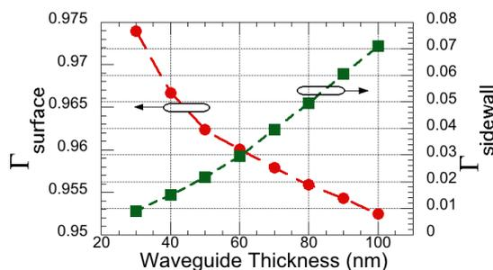
Fig. 2: Dependence of overlap factors on core geometry
