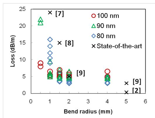
Fig. 3: Propagation losses measured using ring resonators as a function of bend radius. The best results from literature are also shown (black)
