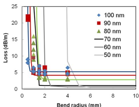
**Fig. 5:** Measured propagation losses (markers) compared to calculated radiation losses (lines) for waveguides having a width of 2.8  $\mu\text{m}$ . The scattering-loss dominated floor is fitted to the data. The 50-70 nm data are simulation results.
