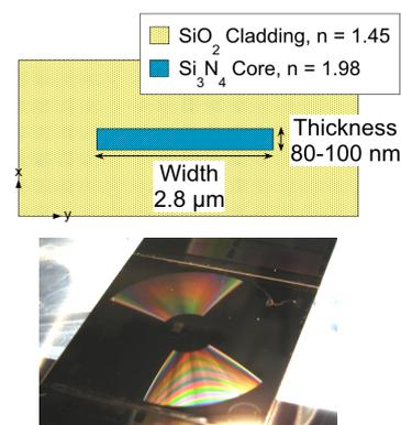
**Fig. 1:** (top) Schematic cross-section of waveguide (bottom) Top-down view of 20-m spiral delay having a footprint of 9 cm<sup>2</sup>.
