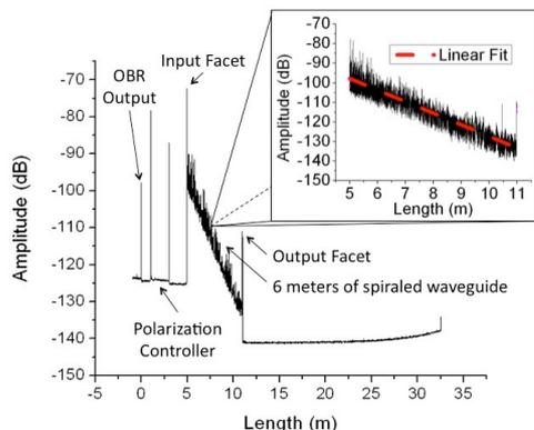
**Fig. 4:** Reflected power data from Luna OBR (inset) linear fit used to determine loss
