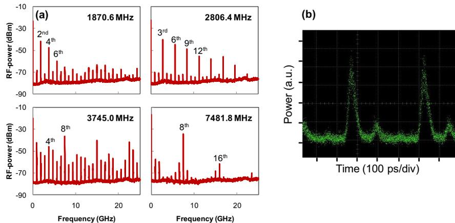
Fig. 4. (a) RF-spectra obtained at 20 dBm injection at the indicated frequency and with a bandwidth of 5 MHz. (b) Time-domain trace obtained at an injection frequency of 2807 MHz.
