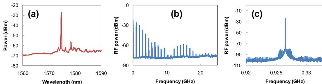
Fig. 2. (a) Optical spectrum at 12 dBm RF-power at 927 MHz. The optical bandwidth used is 0.06 nm. (b,c) RF-spectra obtained at 20 dBm RF-power. The spectrum analyzer resolution bandwidths in (b) and (c) are 5 MHz and 10 kHz, respectively.
