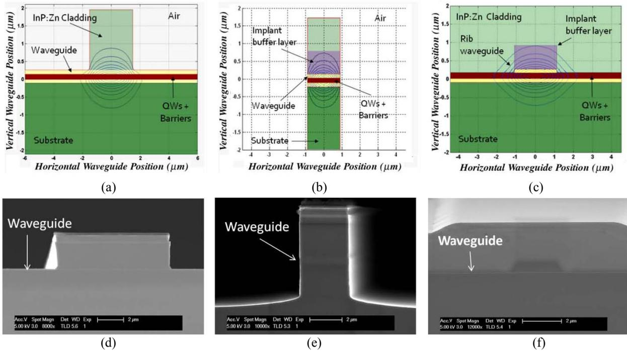
Fig 3. Waveguide architectures used in MOTOR: (a), (b), (c) show schematic cross-sections with the optical mode profile superimposed for surface ridge, deeply-etched ridge, and buried rib, respectively. (d), (e), (f) show SEM cross sections for surface ridge, deeply-etched ridge, and buried rib, respectively
