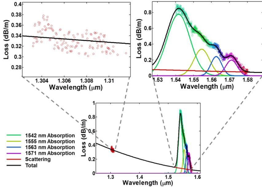
Fig. 2. Propagation loss vs. wavelength for a waveguide with a 40-nm-thick by 13- $\mu\text{m}$ -wide core and bonded thermal oxide upper cladding. OFDR data are averaged over a 50 nm spectral window centered at each marker. The large spectral window reduces the error in measurement, but it also increases averaging of the actual spectral dependence of propagation loss.
