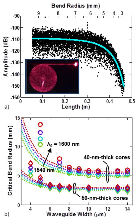
Fig. 1. a) OFDR data used to measure the bending capabilities of planar waveguides. The top horizontal axis shows the dependences of backscatter amplitude on bend radius. The solid line is a nonlinear fit to the data. Data is taken from a spiral structure shown with red laser light in the inset. b) Critical-bend-radius vs. waveguide width for waveguides with 40 and 50 nm thick cores fit at 1540, 1560, 1580, and 1600 nm wavelengths. Dashed lines are simulated values.
