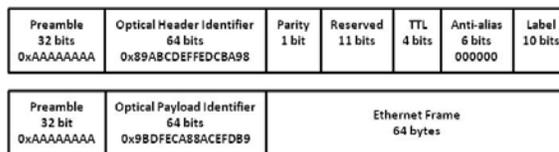
*Fig.1: Optically labeled packet format: 10Gb/s NRZ optical header (top) and 40Gb/s RZ optical payload (bottom).*
