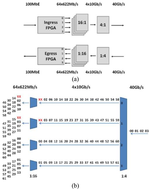
Fig. 2: (a) Adaptation between 100MbE frames and 40Gb/s optically labeled packets. (b) Non-ideal deserialization of a 40Gb/s serial stream.
