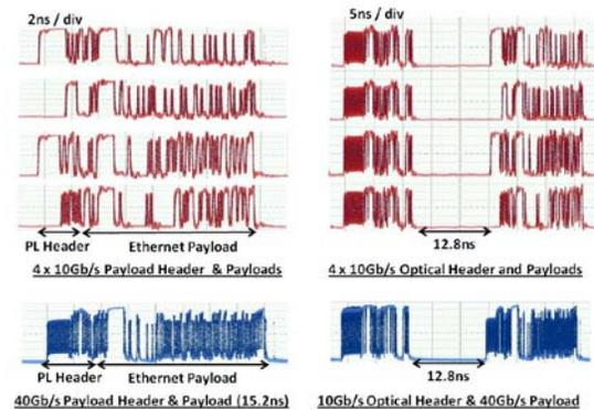
Fig. 3: Oscilloscope traces of the channel-encoded 10Gb/s optical header and 40Gb/s payload at each serialization stage.
