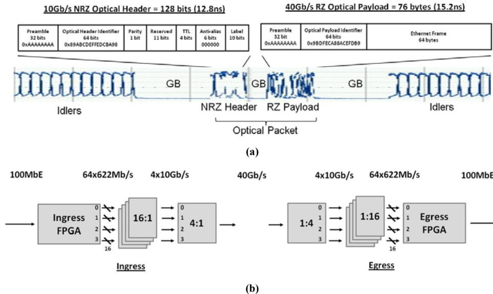
Fig. 1. (a) Optically labeled packet format and (b) de/serialization stages used to achieve adaptation between 100MbE frames and 40Gb/s optically labeled packets.
