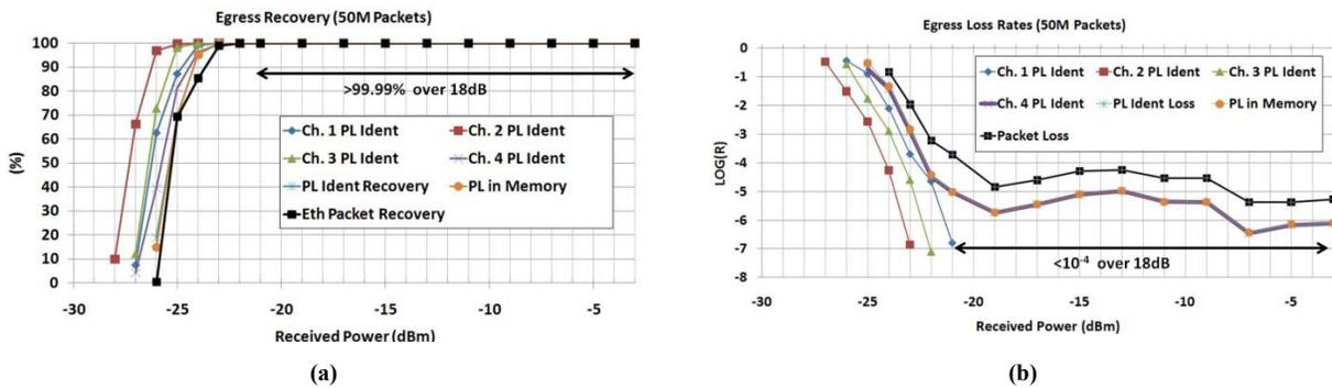
Fig.3. (a) Experimental results showing egress recovery and (b) loss ratios.
