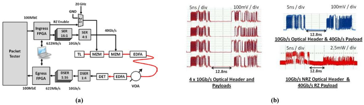
Fig.2. (a) Experimental setup (Packet length = 64 bytes, stream length = 50M packets, IPG = 0.96 $\mu$ s,  $\lambda$  = 1550nm,  $P_{TX}$  = -3dBm) and (b) oscilloscope traces of optically labeled packets at different ingress stages of serialization.
