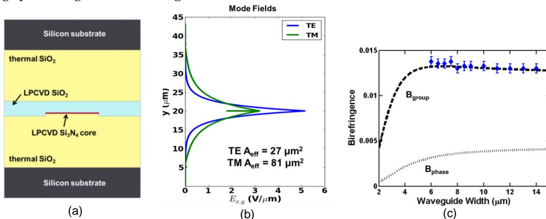
Fig. 1. a) Cross-section of waveguide structure and b) simulated fundamental TE and TM modes for a 7- $\mu\text{m}$ -wide core at  $\lambda_0 = 1.55 \mu\text{m}$ . c) Calculated group and phase birefringence with measured values for various core widths.
