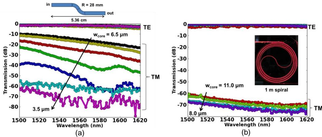
Fig. 4. a) Polarization extinction measured in a single s-bend of 28 mm bend radius for different waveguide core widths and b) polarization extinction measured in a 1 m spiral delay line for various core widths.
