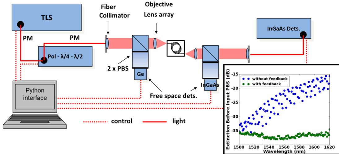
Fig. 2. A schematic of the setup used for the measurement of high polarization extinction. "PM" indicates polarization maintaining fiber. The inset shows how feedback is necessary to maintain high input polarization extinction during the wavelength sweep.
