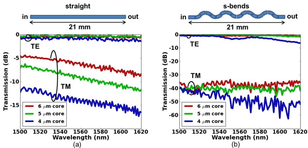
Fig. 3. a) The polarization extinction measured in straight waveguides and b) a series of R = 9.8 mm s-bends.
